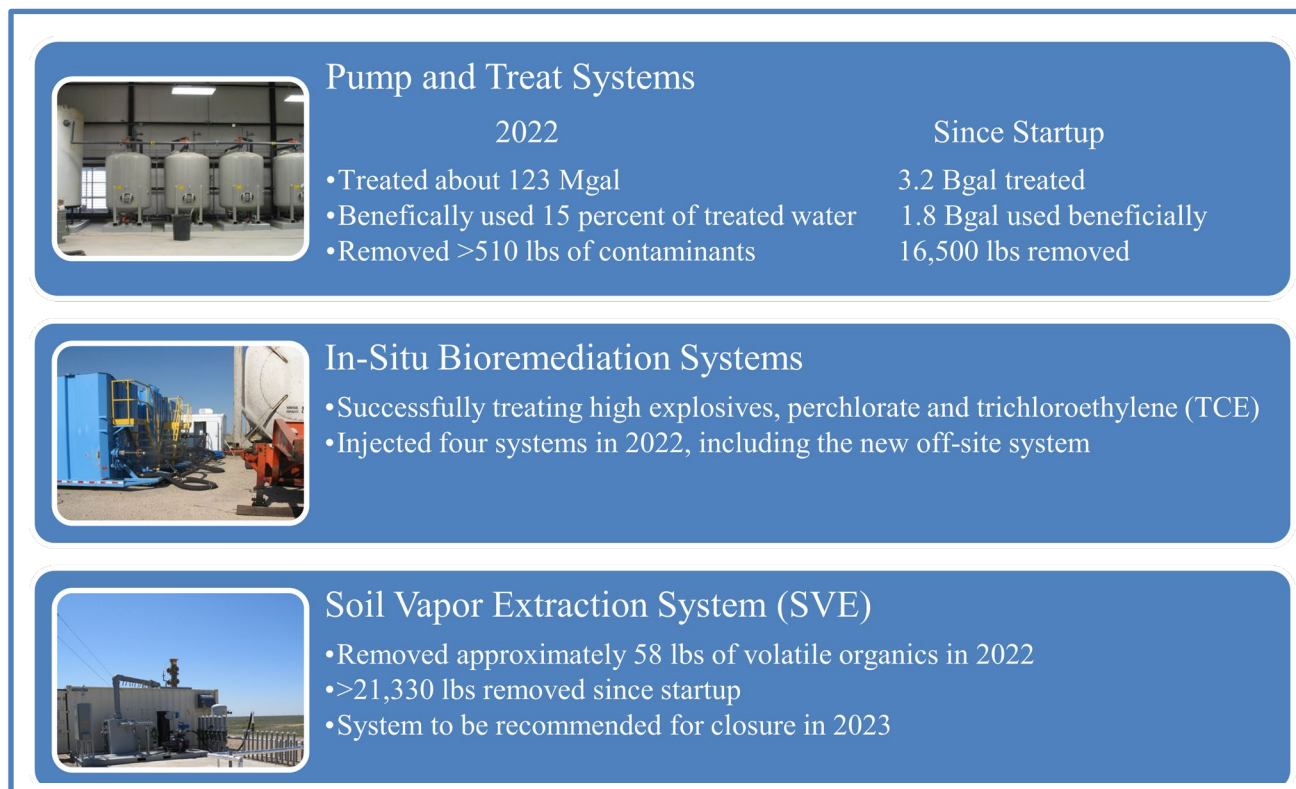
Fig. 3.6. Major Milestones for 2022 Remedial Actions
