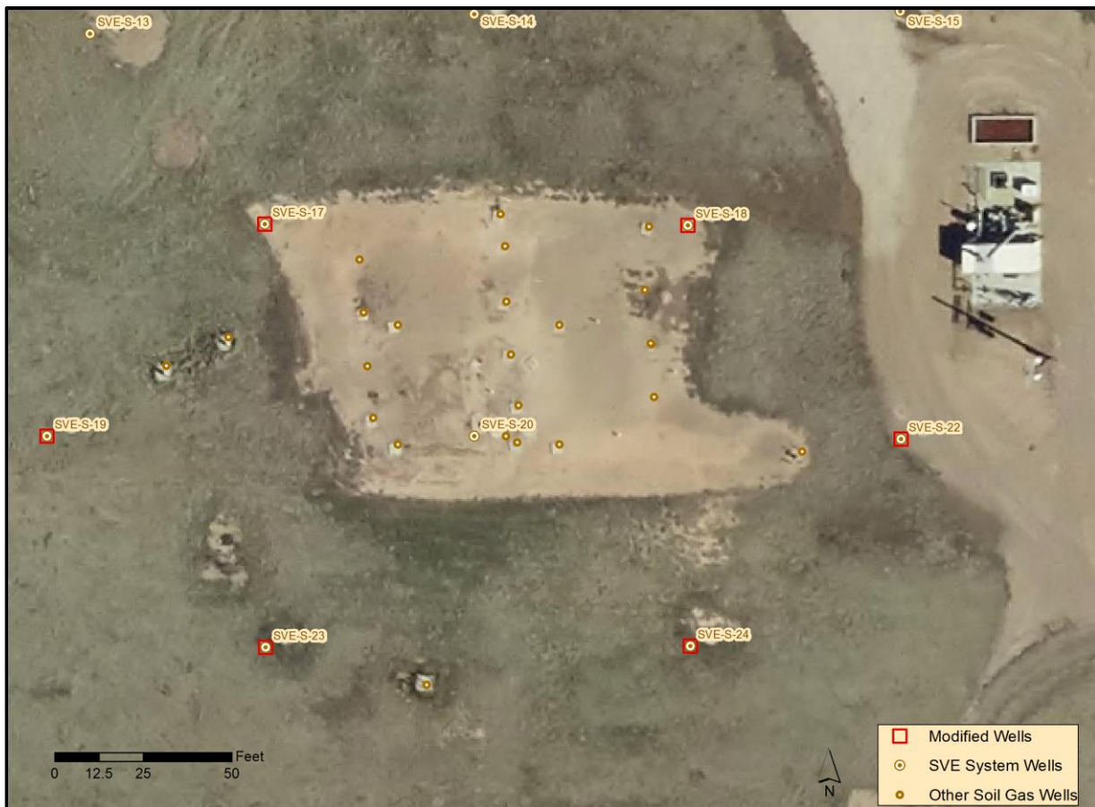
Fig. 1-4. Burning Ground SVE System wells and modifications.
