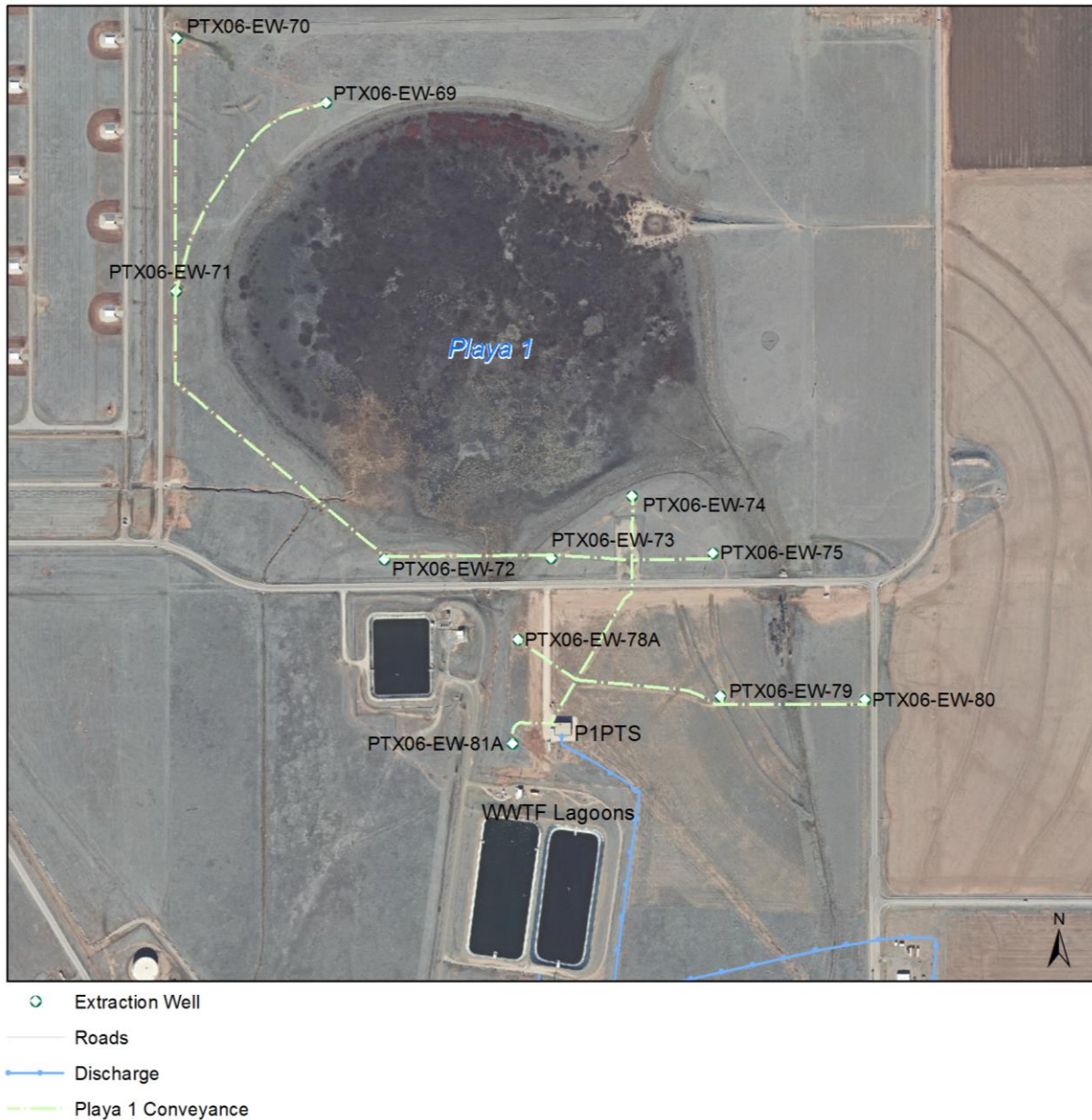
Fig. 1-6. P1PTS wells and conveyance lines.
